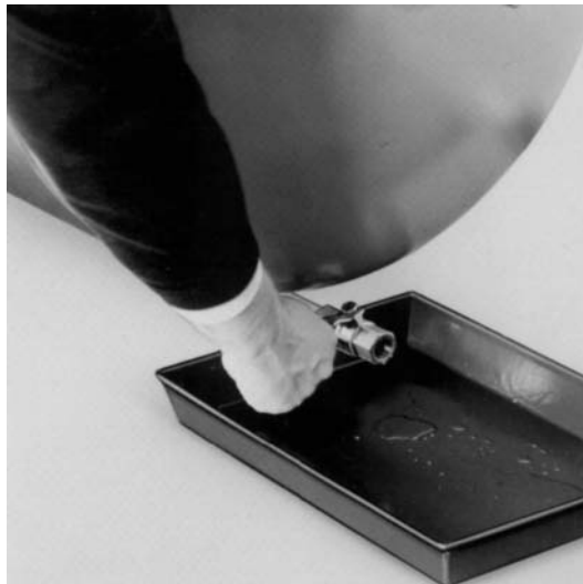
Fig. 5.2: Draining off the condensate manually
