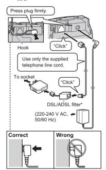
\*DSL/ADSL filter (not supplied) is required if you have DSL/ADSL service.
