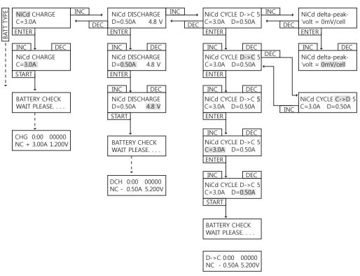
NiCd CHARGE C=3.0A Setting charge current
