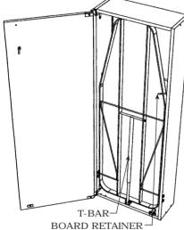
To open Ironing Board, lift retainer and pull down as shown in diagrams.
