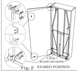
Locate and fix hinge brackets to cabinet with 2 large screws provided.
