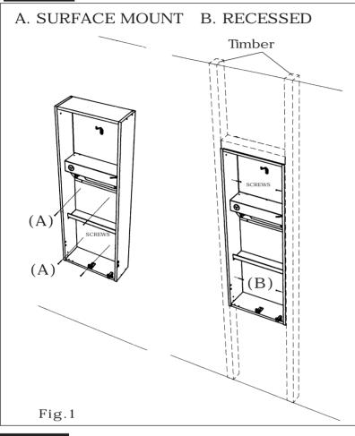
The ROBINHOOD Ironing Centre can be mounted in two ways (Fig1) a) Surface Mount - make sure solid timber studs or mounting points are in a suitable position for the mounting of the Ironing Centre. Drill and fasten through the back of the wooden panel only to the Mounting Points (A) with the 4 screws supplied (it may be necessary to purchase different length screws for correct fitting, or use wall anchors if unit is to be mounted to a solid wall).
