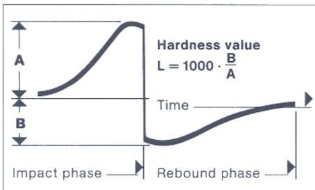
This hardness value is a 3 digit value; the harder the tested material, the higher the "L" value. The L value is additionally designated with the identifying letters of the impact device.
