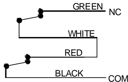
SERIES CONNECTION OF SWITCH AND TAMPER NC LOOPS TO MAINTAIN BOTH FEATURES WITH A SINGLE ALARM POINT.
