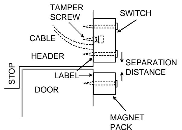
Drill 7/64" (2.75MM) diameter pilot holes for the #8 mounting screws.
