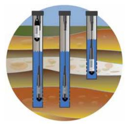
data must be used to compensate the pressure measurements recorded by the Divers for variations in atmospheric pressure. A Baro-Diver, designed for taking atmospheric pressure measurements, is recommended for this purpose. In principle, a single Baro-Diver is sufficient for an area with a radius of 15 kilometres (depending on terrain conditions. Also see Appendix II 'Use of Divers at Elevations').
