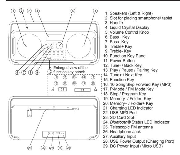
The FREESTYLER JR runs on an internal rechargeable Lithium-ion battery. Press the **POWER** button to switch the unit on.
