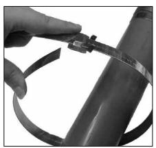
1. Band may be used from bulk roll as this completely eliminates waste of band. Slide buckle on band as shown, bringing end of band around object to be clamped and again through buckle.
