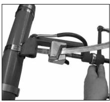
5. Roll tool over buckle, backing off with tension handle1- 1½ turns throughout entire rolling operation. Failure to back off tension with tension handle throughout entire course of roll-over may result in breaking of band. There is no loss of tension as band released is used up in the bend.
