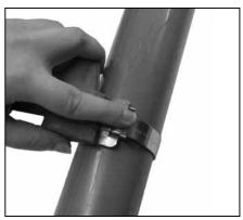
4. Place finger on BAND-IT Band at buckle bridge while tensioning with tool handle. When you feel BAND-IT Band stop moving through buckle as you are turning handle, maximum pressure is being exerted by the BAND-IT Band around object being clamped. Stop turning handle.
