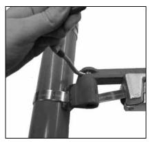
6. Pull cutting handle to cut the band. When applying Giant Band clamps, prior to cutting off clamp, release band gripper and push tool nose away from buckle approx. 1/4".
