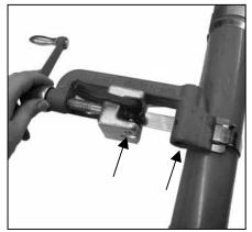
3. Place band in open of tool nose and gripper block. Move into slot as far as possible, to avoid buckle sliding into tool nose. Apply tension by turning handle of tool
