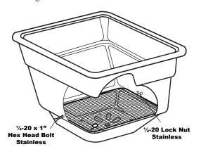
19. Install debris screen into hopper, then insert 1/4-20 x 1" Stainless Steel Hex Bolt thru the hole in the side wall of the hopper. Secure with Stainless Steel lock nut - TIGHTEN WITH HAND TOOLS ONLY
