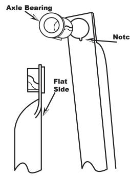
**5.** Install axle bearings to both lower handles. **NOTE:** Notch on bearings and lower handles. Bearings must go through flat side of lower handle.
