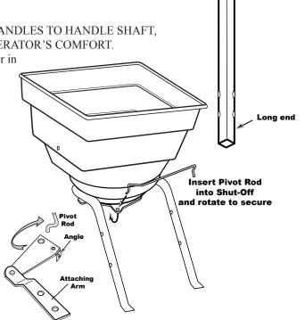
**13.** Install handle shaft to lower handles and pivot & bracket assembly as shown. Using 1/4-20 x 2" bolts and (as shown) and locknuts. **TIGHTEN BOLTS AND NUTS NOW.**
