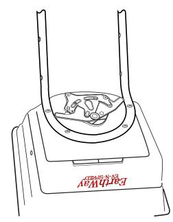
**4.** Install gear box by inserting the pinion shaft into hole in center of hoppers bottom. The word "FRONT" on the gearbox must point to Front of the hopper. Follow label instructions on hopper.
