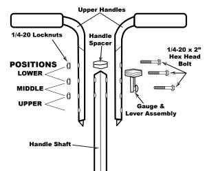
10. NOTE: BEFORE INSTALLING GAUGE AND UPPER HANDLES TO HANDLE SHAFT, UPPER HANDLES FEATURE THREE POSITIONS FOR OPERATOR'S COMFORT.
