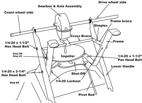
**6.** A - Install lower handles onto axle to both sides as shown. Insert 2½" bolt through second hole in lower handle and through first hole in frame and install locknut. **DO NOT TIGHTEN.**
