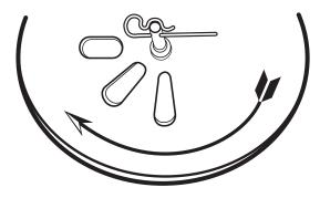
**18.** Insert agitator to pinion shaft on inside of hopper. **Note:** the position of flat side of the agitator. This pin should be installed as shown.
