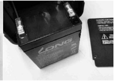
Be sure to connect battery correctly Red = + positive Black = - negative
