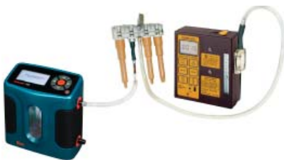
Connect holder to pump intake and tube inlet to calibrator.
