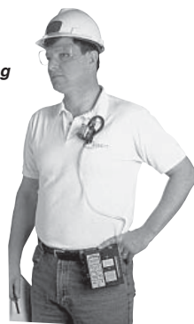
Clip sample medium to worker and pump to belt.
