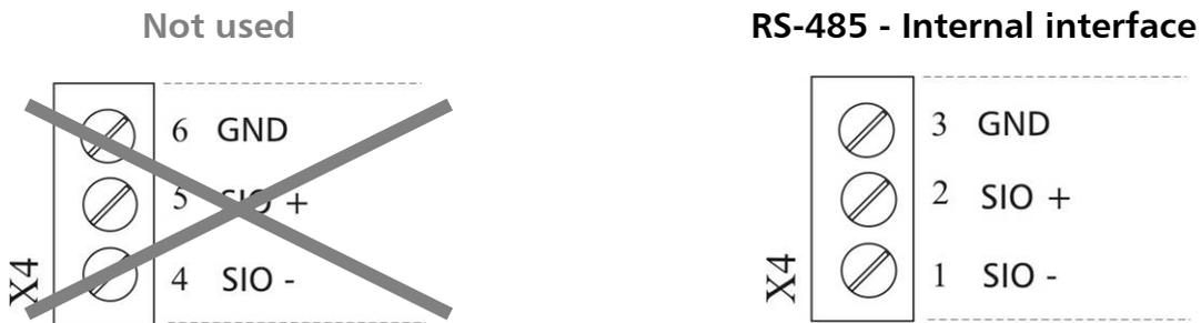
The **internal RS-485 Interface** is used for the communication between up to 4 HYDROVAR units in a multi-pump application. For the connection of each HYDROVAR via the RS-485 interface the terminals X4/1-3 on the control card (HV2.015-4.220) and either the terminals X5/1-3 or X6/1-3 on the control card (HV2.1-3.22) have to be used.
