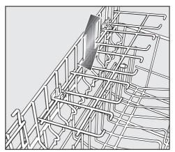
Slide the glass rack to the desired height until the catches click into place at the top.
