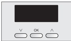
The display is operated using the  $\lor$ , **OK** and  $\land$  buttons. The value or option currently selected will appear highlighted.
