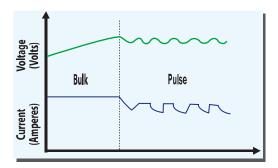
**Bulk:** This is the first stage where the battery is in a low charge state (typically 10%), & receives the majority of its charge. During this stage the battery is brought to about 95% of its charge by getting 100% of the available solar power.
