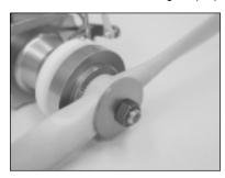
Running your engine using an out-of-balance propeller can lead to excessive vibration, which will result in excessive stress and wear on both the engine and the airframe. Balance the propeller using the method recommended by the propeller manufacturer. Several products are available to properly balance propellers. Ask
