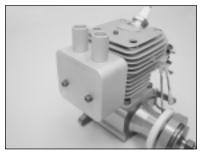
The muffler is mounted to the engine using the two steel socket-cap screws, two split washers and the gasket provided. To prevent the muffler screws from loosening during flight, apply blue threadlock to the screws before installing them. Also make sure to tighten the screws firmly.
