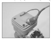
end of the spark plug until it snaps down into place. To ground the ignition system, secure the grounding wire to the top of the cylinder head using the socket-cap screw, as shown. Now plug together the ignition lead from the engine and the ignition lead from the ignition module.
