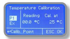
Note: This procedure assumes that instrument is correctly configured and properly connected to a working PT100. Calibrate using plant's temperature otherwise unattended results may occur.
