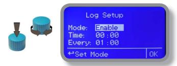
Log activity recording can be started by moving wheel on "Mode: Disable" and changing it to "Mode: Enable". Log activity starting time can be set to begin at specified time by entering "Time". Activities data are collected every specified hour or minutes. Edit this parameter by moving wheel on "Every: 00:00" and changing it to desired time.
