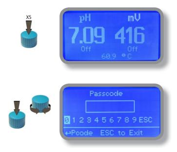
To set a new passcode choose "PARAMETERS" from "Main Menu", move on "New Pcode", click on wheel and enter a four numbers code. Click on "EXIT" and choose "YES" to save request. The new passcode is now ready.
