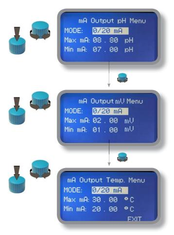
Rotate wheel to move within all 3 channels. Click wheel to selecte parameter and rotate wheel to change it. Click wheel again and rotate wheel to move cursor on next parameter. To end procedure move cursor on "EXIT" and press wheel to proceed to "Save" request screen. Move wheel on "YES" to save or "NO" to discard changes.
