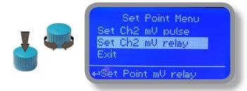
Proportional mode set the instrument to operate using a calculated percentage between two set values that enable or disable the ORP pump. To use this mode move cursor on "Working Mode". Press the wheel and select it.
