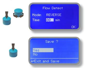
To end procedure move cursor on "OK" and press wheel to proceed to "Save" request screen. Move wheel on "YES" to save or "NO" to discard changes.
