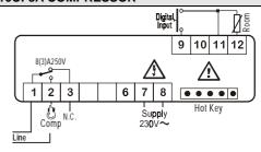
12Vac/dc supply: connect to the terminals 7 and 8. 24Vac/dc supply: connect to the terminals 7 and 8. 120Vac supply: connect to the terminals 7 and 8.
