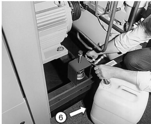
Fig. 6.12: Drain off old oil from oil/compressed air receiver
