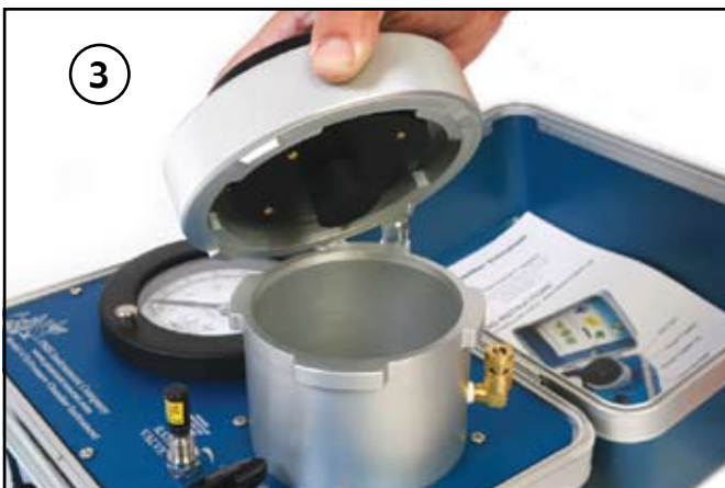
Install the lid on the chamber
