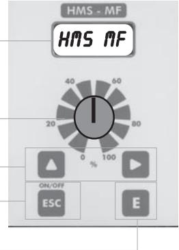
The “HMS MF” pump is equipped with a keyboard. To avoid any misunderstanding during next chapters all keys will be described as shown on this legend:
