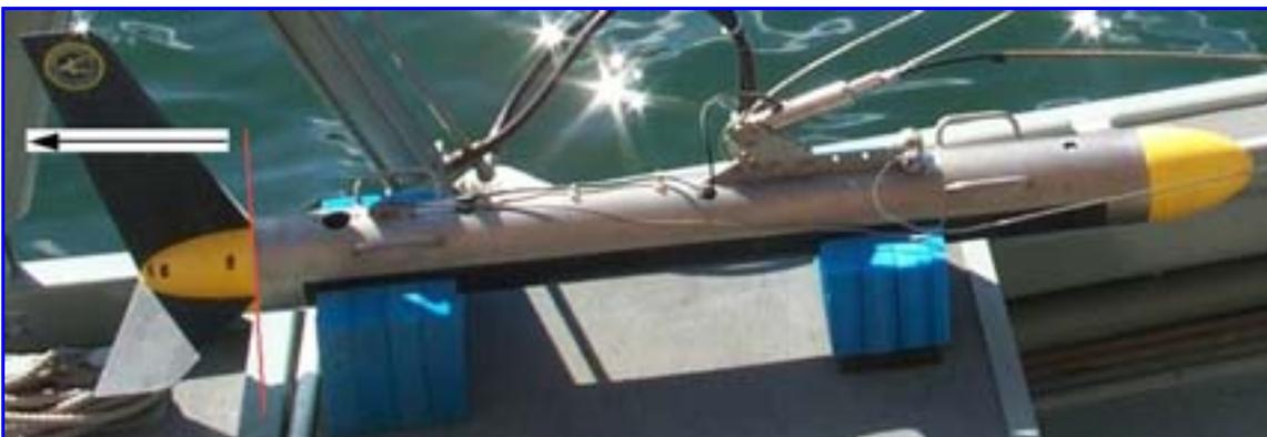
*Figure 18 The Klein 5500 sidescan sonar showing where the rear yellow nose cone, housing the tail fins, will separate (indicated by a red line) from the stainless steel body when the tail fins become snagged on any bottom objects.*
