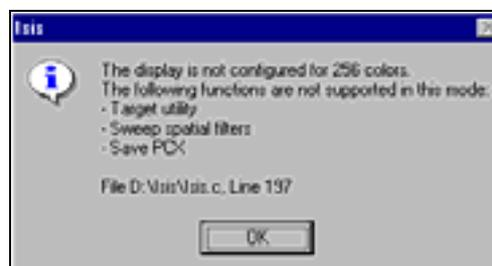
Figure 41 The error spawned by the Isis<sup>®</sup> software, version 4.54, when the colour depth has not been set to 256 colours.
