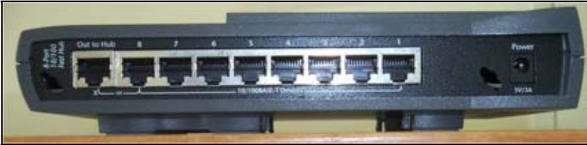
Figure 25 The back of the Intel In-Business hub, showing the "X" RJ45 input slot, which accepts input data from a cross-over cable.
