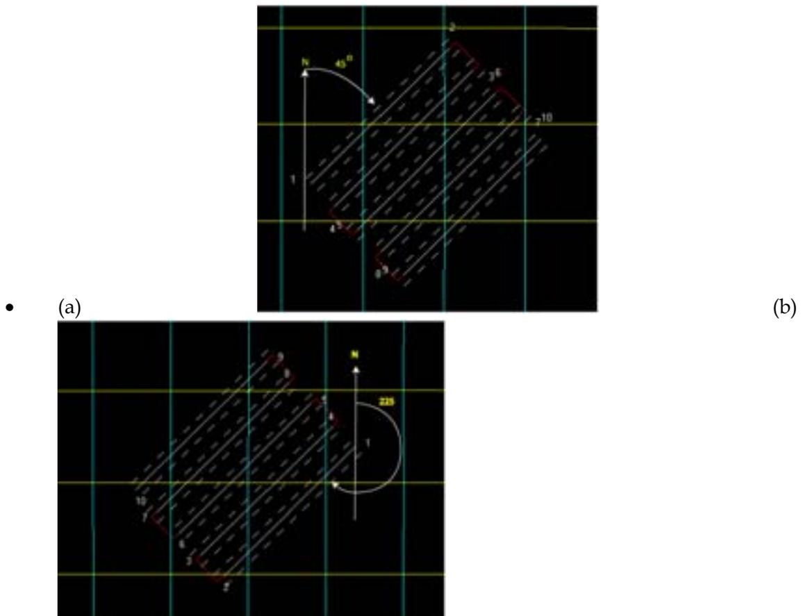
Figure 73 Two examples of 5 survey lines created with line headings of (a)  $45^{\circ}$  and (b)  $225^{\circ}$ , respectively. In both examples the origin (as needs to be entered into the survey route dialogue box) is at the waypoint #1, although because of the difference in line heading this origin appears in opposite places of the survey grid.
