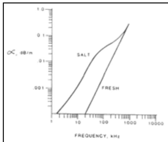
Figure 2 The empirical relationship determined by Francois and Harrison (1982) between the absorption coefficient of acoustic energy and frequency for fresh ( $10^{\circ}C$ ) and saltwater ( $10^{\circ}C$  and 35parts per thousand).
