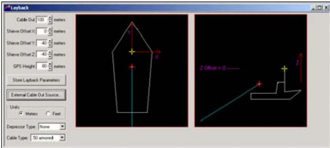
Figure 69 The Layback dialog box used in SonarPro.
