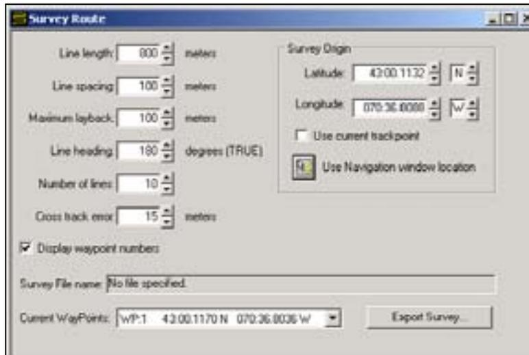
Figure 72 The survey route set up dialogue box used in SonarPro.
