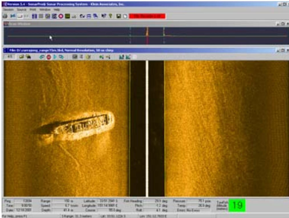
Figure 88 Waterfall display of the Klein 5500 showing streaking.
