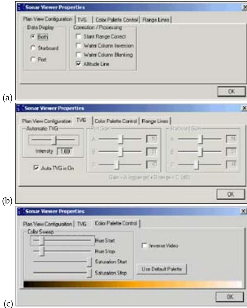
Figure 84 The three tabs of the Sonar Viewer Properties window. (a) Plan View Configuration, (b) TVG and (c) Color Palette.
