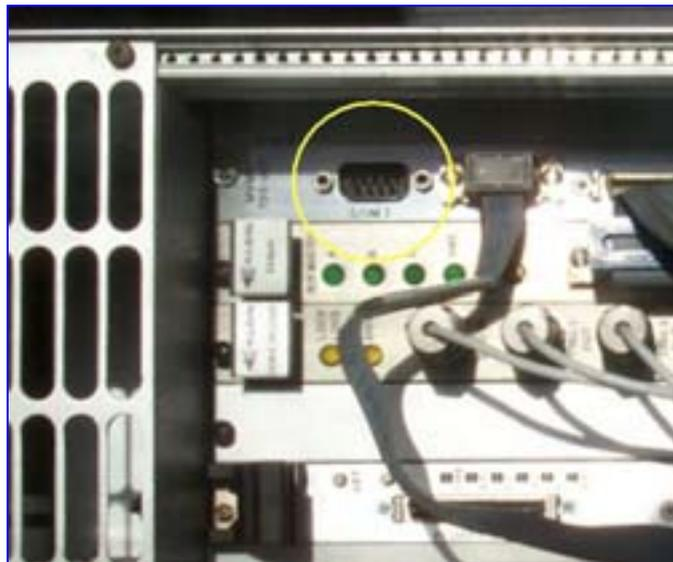
Figure 44 The Front panel of the TPU showing the Com1 serial input port (marked with a yellow circle).
