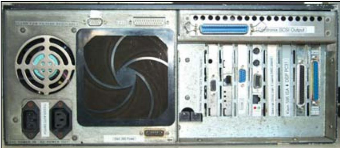
Figure 22 The back of the Isis ruggedised computer.
