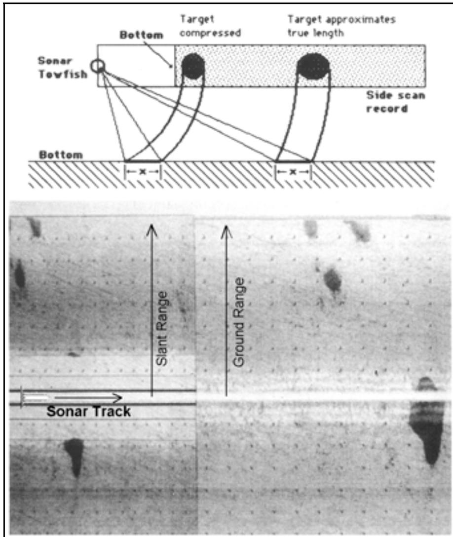
Figure 5 A schematic showing the across track compression that occurs in waterfall displays when backscatter levels are displayed versus slant range and how this compression can be circumvented by displaying backscatter levels versus ground range and not slant range. Adapted from Klein (1985).
