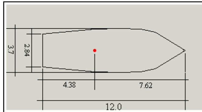
Figure 27 Schematic diagram of the DSTO workboat "440", showing the major length and width attributes (in metres) in comparison to the GPS antenna (marked by the red dot).
