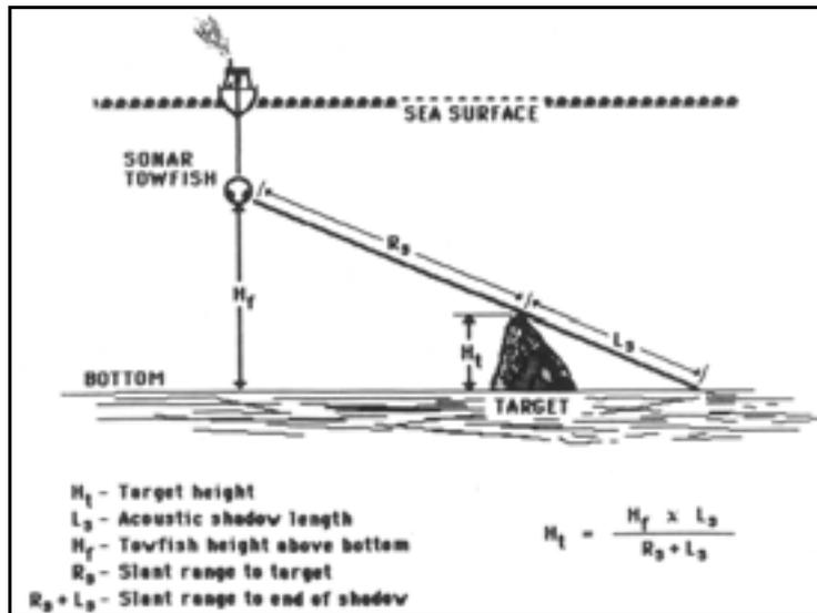
Figure 12 A schematic diagram of a sidescan's cross track geometry showing how a target's height above the seafloor is calculated. Taken from Klein (1985).
