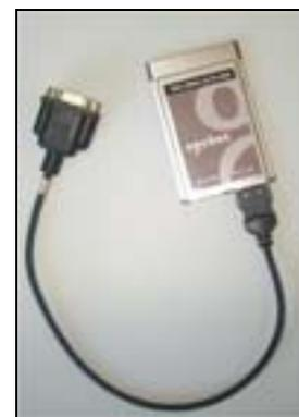
(a) Digiboard Classic, 8 serial port PCI card. (b) Dual serial PCMCIA card from Socket Communication ([http://www.socketcom.com/product/serial\\_dual.htm](http://www.socketcom.com/product/serial_dual.htm)).
