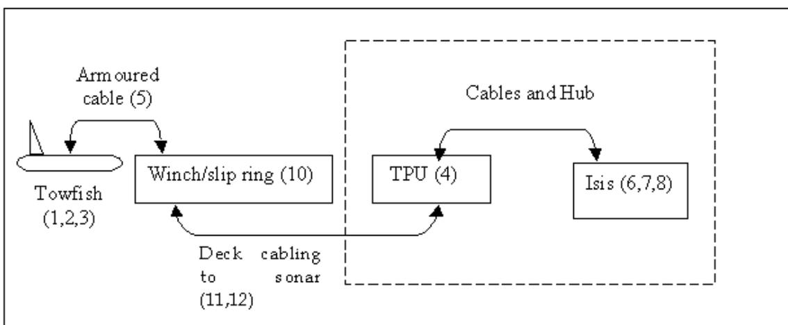
Figure 21 A flow diagram showing the hardware setup for the Klein 5500 sidescan sonar.
