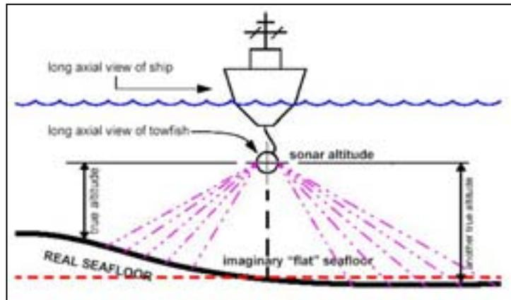
Figure 85 A schematic diagram showing how the flat bottom assumption can result in incorrect location of objects in areas of uneven bottom topography.
