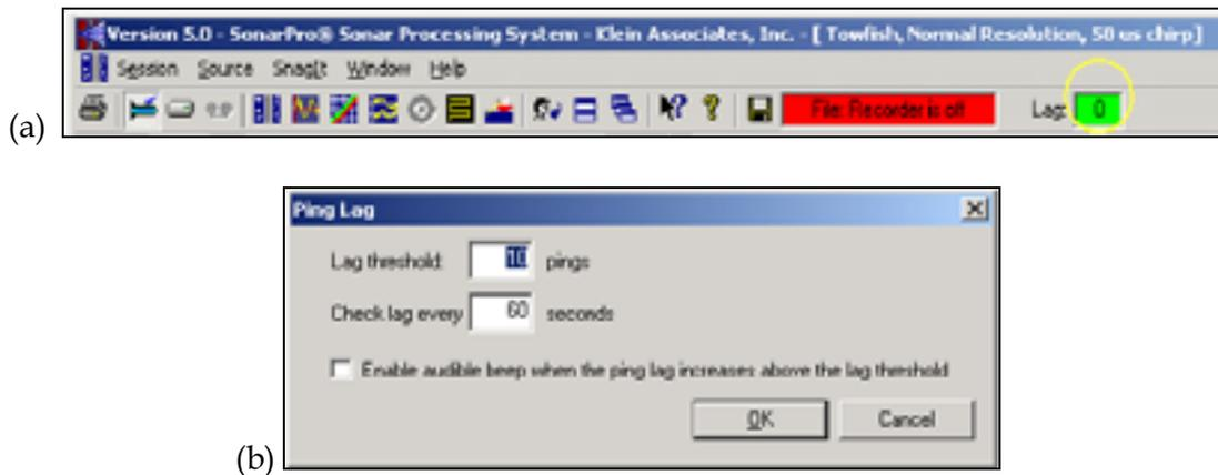
Figure 68 (a) The top portions of the main window, in particular showing the Lag status window on the right-hand side (circled in yellow). (b) The Ping Lag dialogue box.
