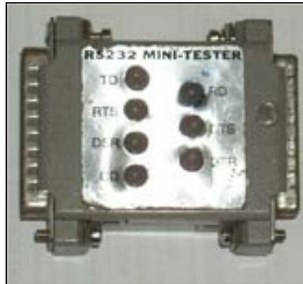
Figure 87 The RS232 Mini Tester from Jaycar.
