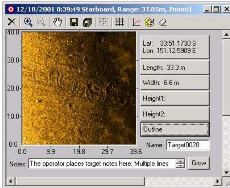
Figure 71 An example of the Target window in SonarPro. In this example the Target window is displaying the characteristics of an old chain located beneath the Sydney harbour Bridge.
