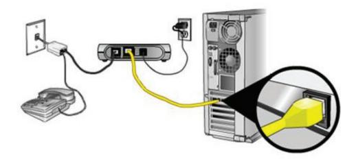
5. Disconnect and reconnect the ADSL cable at both ends and the filter to make sure it is **not loose**.
