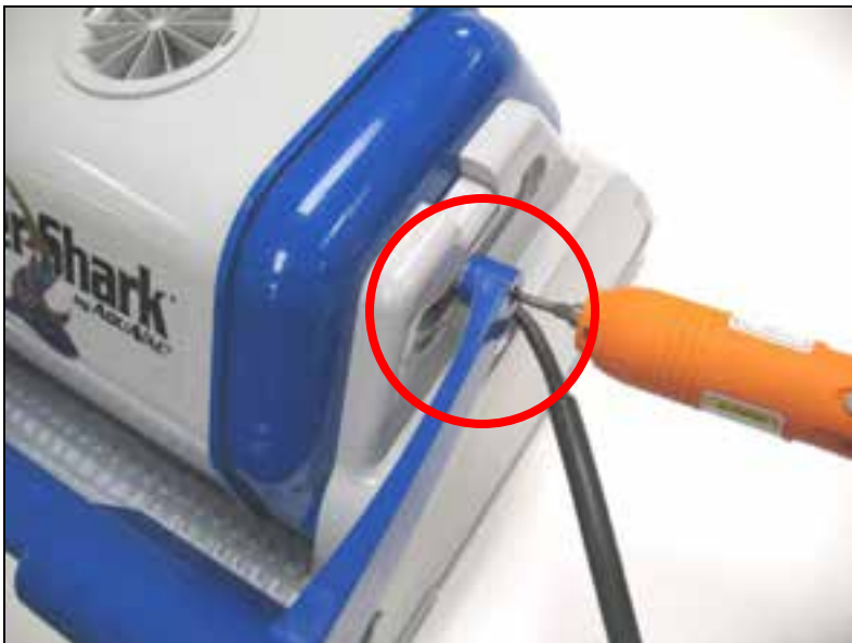
Handle removal 1 screw each end
