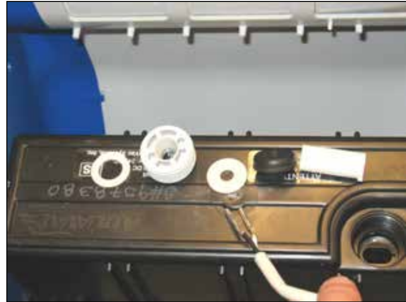
Connector, seals and washers removed.
