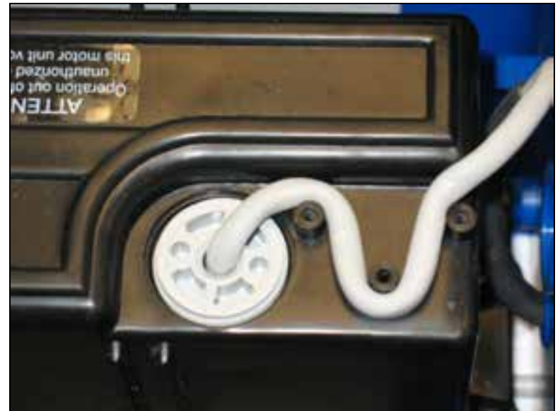
Plate removed showing strain relief system.
