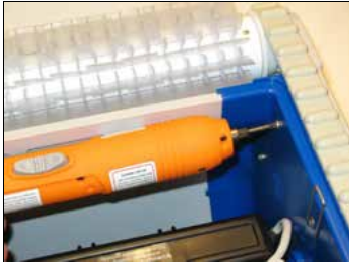
Screw removal, opposite side cover, non-drive side.
