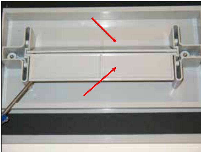
Inlet flaps, check for free movement.
