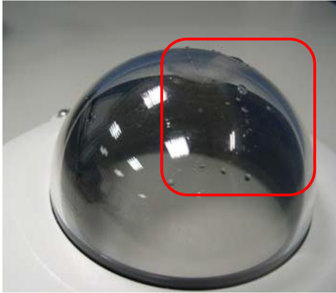
IR reflection caused by fogging of the cover
