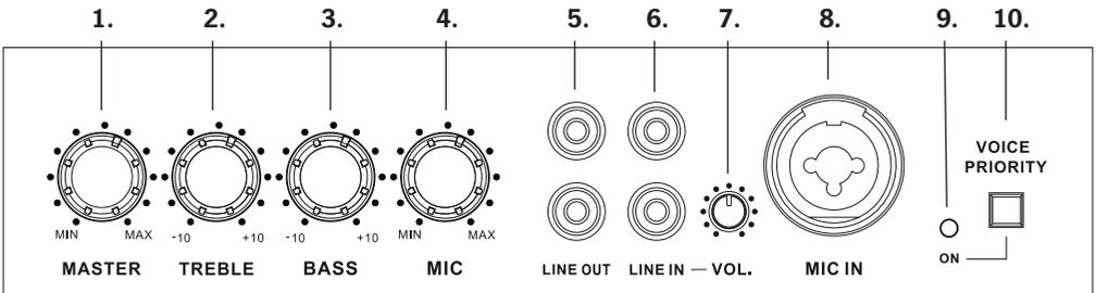
**Figure 4: Level Adjustment & Input/Output Module (Models C 7185B)**
