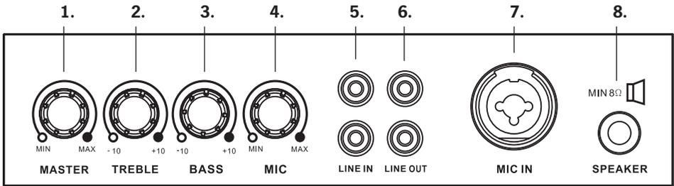
**Figure 3: Level Adjustment & Input/Output Module (Models C 7180, C 7182B and C 7184B)**
