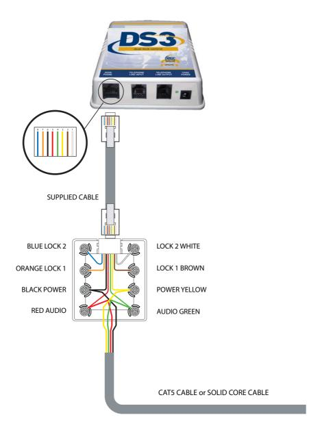
The colours used are those of the wires in the supplied Interface box.
