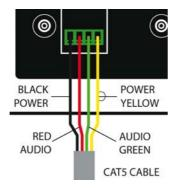
Two wires are required for the AUDIO SIGNAL and Two wires are used to provide POWER to the unit.
