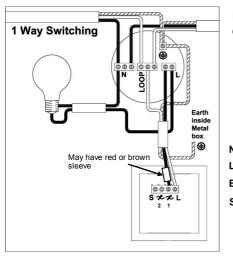
If the lights are controlled from one location only, wire as in the diagram.
