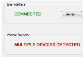
Both the link from PC to Line Interface Card (LIC) and the iStud Bus are operational, however more than one Vehicle Detector is connected to the iStud Bus.
