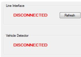
The link from PC to Line Interface Card (LIC) is not working.
