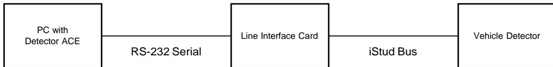
A standard RS-232 serial COM port is used on the host PC for the connection to the Line Interface Card. If the PC does not have a built-in serial port then a USB serial adapter can be used. This connection is labelled 'COMMS' on the Line Interface Card and uses an RJ-45 to DB-9 cable.
