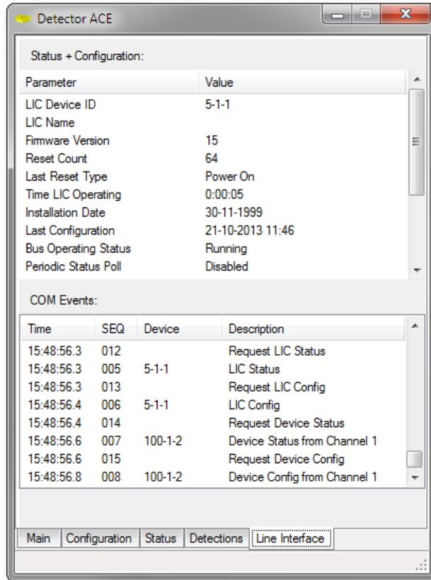
The Line Interface tab can be helpful in diagnosing communication problems. It is divided into two sections. The upper section shows a number of internal parameters from the Line Interface Card, while the lower section shows the messages being sent and received on the RS232 serial interface. You may be asked to provide a copy of this information when calling for technical support.
