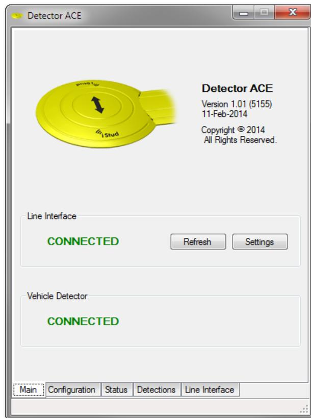
It also has two Line Interface action buttons which allow the link parameters to be adjusted. Their operation is described in section 2 above.
