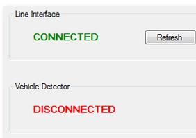
The link from PC to Line Interface Card (LIC) is working; however the iStud Bus between the LIC and Vehicle Detector is not operational.
