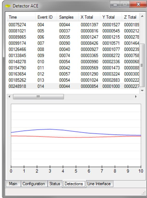
The Detections tab can be helpful in diagnosing vehicle detection problems. It shows summary information along with magnetic waveform images for vehicle detection events.
