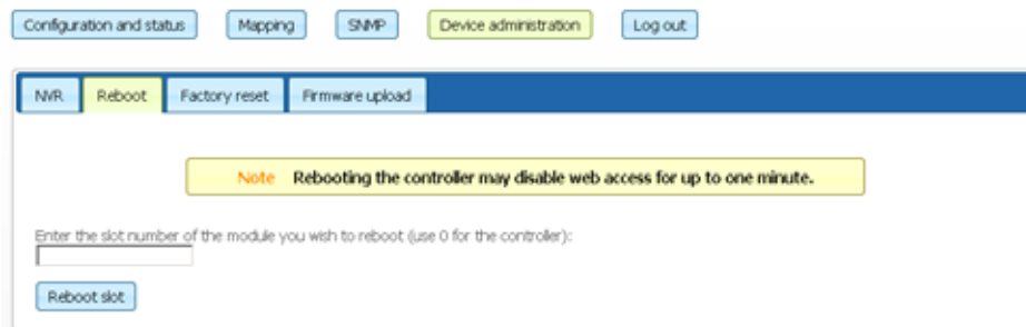
Figure 31: The Controller/TAP module reboot screen
