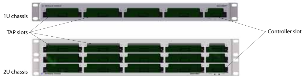
Figure 8: Location of the TAP and Controller slot
