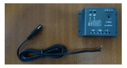
The other lead in the kit which has two bare wires is used with the 5 amp regular.
