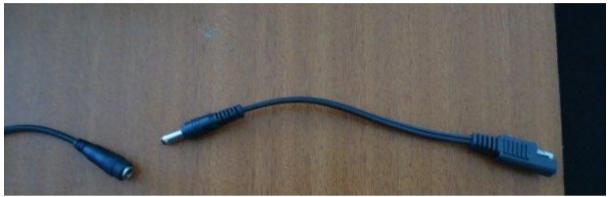
Plug this lead into the 5m solar panel lead. This lead is used for charging the phone and the laptop.
