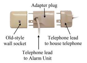
Remove the house telephones lead from the wall socket and plug-in the large adaptor plug.
