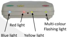
Switch-on the power on the rear of the Alarm Unit and check the lights flash on the front panel.
