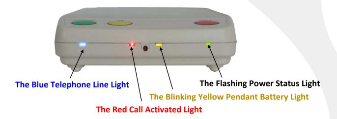
The lights on the front of the FirstCall alarm show the operational status of the equipment, and if a problem has been detected.
