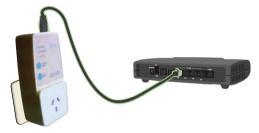
Connect the other PG-9022 to your fetchtv Set Top Box, computer, V-box or other network device using an Ethernet cable. This is the End Point (EP).
