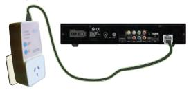
Shortly, you will see the Ethernet LED blinking; this indicates that there is data traffic going through the PG-9022. You are now ready to start using your network.
