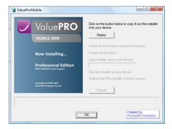
Press the [Deploy] button. The installer will automatically check your device via the USB cable and start to transfer the software to your phone for you. It will also explain to you that you must click [OK] on your phone to allow the installation to proceed.
