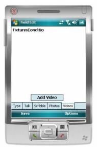
Pressing [ Add Photo ] or [ Add Video ] will start the device's on board camera. Use the [ Camera ] button on your device to snap a photo, or for a video, press the [ Camera ] button once to start recording, then zoom and pan and even talk if you wish to record audio with the video clip, then press the [ Camera ] button again to end the recording.
