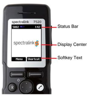
The display is divided in three parts: Status bar, Display center and Softkey Text (see figure above).
