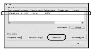
The SmartWizard GearDiscovery utility finds the switch and displays its MAC Address, IP Address, and model number. If you cannot configure your switch, verify that the cable connections are secure, that the IP address configuration of the PC is in the same subnet as the switch, and click the Discover button.
