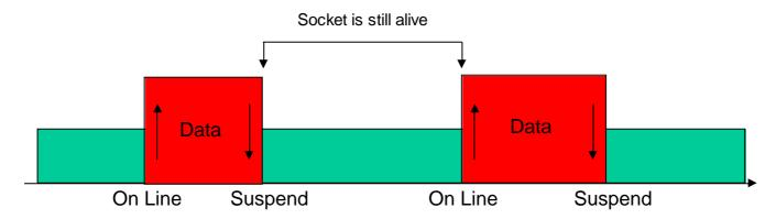
This new feature allows users to switch between online mode and command mode without closing the connection and eventually opening another socket (or resuming the suspended one) or FTP connection.
