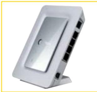
**Step 3 – Connect white Power Cable to the Telephone socket on InZone device (bottom socket), plug the Power Adaptor into a Power Point and check that the signal is green.**
