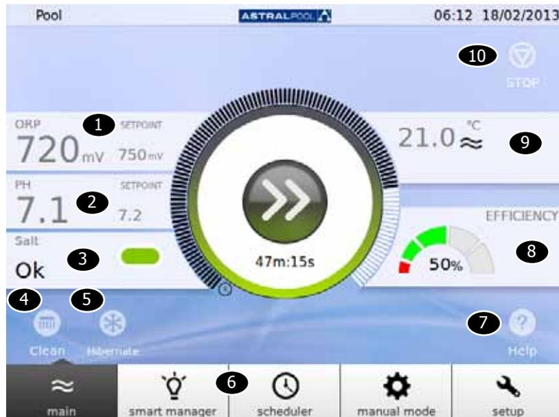
Figure 6: Expanded main screen
