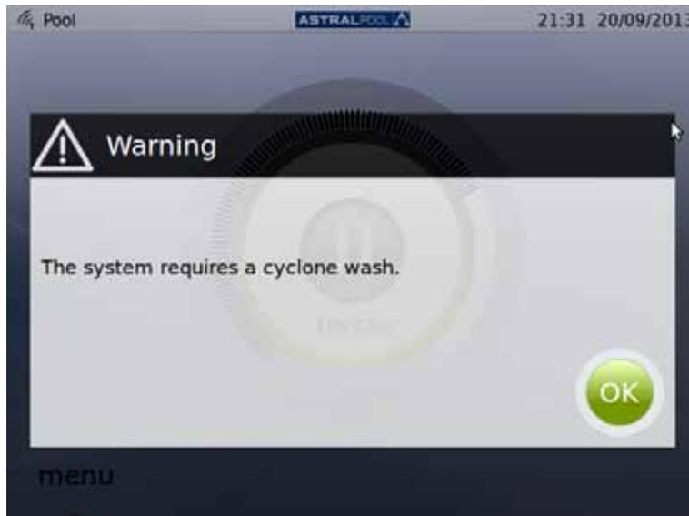
Figure 44: The cyclone needs to be cleaned
