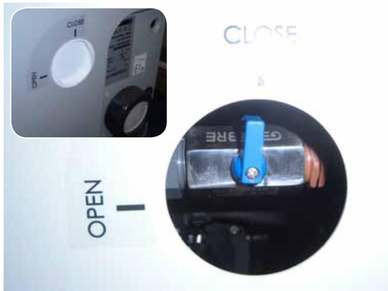
Figure 47: Open the cover and turn the key to the "Open" position.
