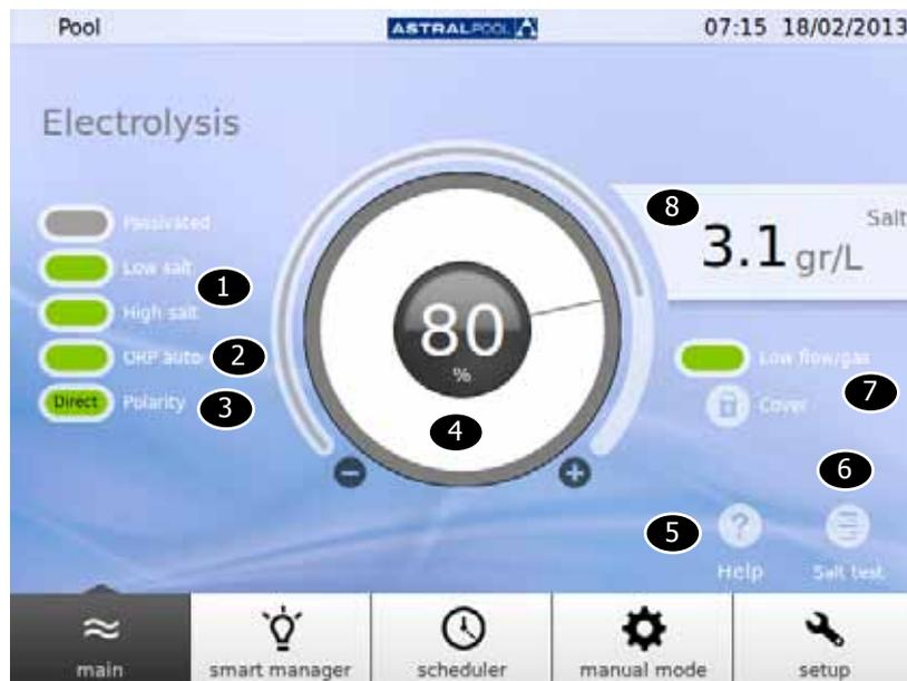
Figure 17: Electrolysis setup
