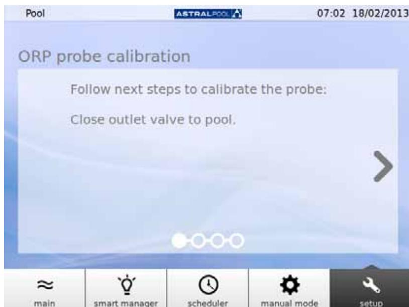
Figure 33: Close outlet valve to pool
