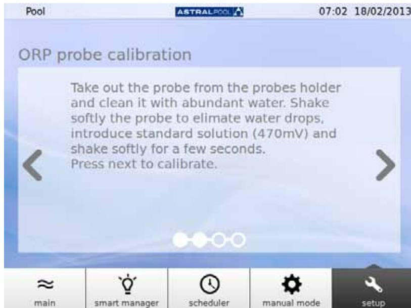
Figure 34: Introduce standard solution
