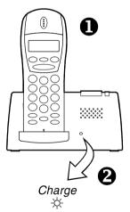
Sit the handset into the handset recess in the base station. ② The correct seating of the handset is confirmed by the phone emitting two beeps. The base station provides visual indication by illuminating the charge LED. Handsets must be charged for 16 hours before first use.
