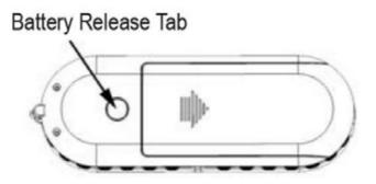
2. Install 4 C-cell batteries (Alkaline batteries recommended) and refit the battery cover.
