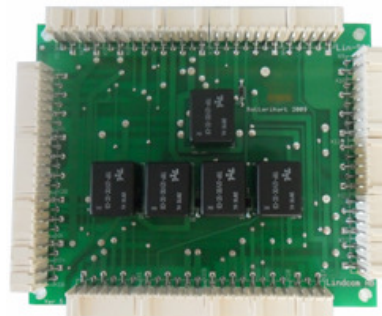
Power Distribution Board
