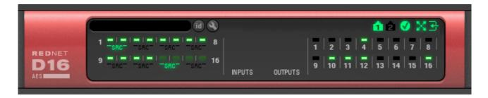
The illustration above shows a RedNet D16 with 16 input signals (SRC switched in for channels 1–2 and channels 13–14) and signal present on five outputs.
