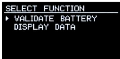
Select the **VALIDATE BATTERY** option from the **SELECT FUNCTION** menu, confirm with '**OK**' and wait for the function to initialise.
