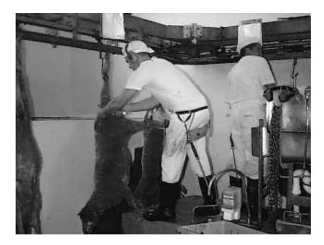
Figure 42: Cutting the animal during the legging task
