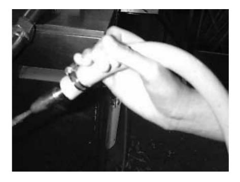
Figure 17: The old hose design (with no cover). Metal elements of the hose end heat up and burn the operators hand
