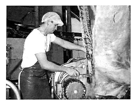
Figure 4: Counterbalancing tools can support the tool weight and Reduce muscular fatigue (Figure courtesy of South Burnnett Meat works).
