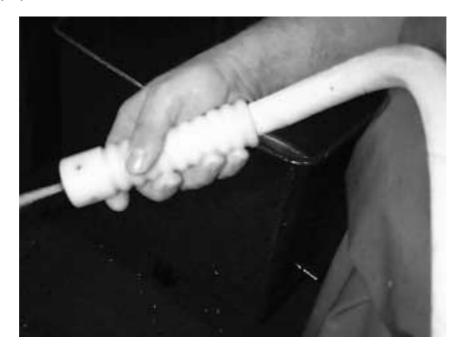
Figure 15: Attachment on the end of the hose. Provides a more comfortable grip on the hose and keeps the hand away from the hot water, and hot metal edge on the hose
