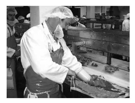
*Figure 9: Using a string to pull the rib away from the meat. Arm only part way through action. Elbow comes up to arm pit height at end of movement*
