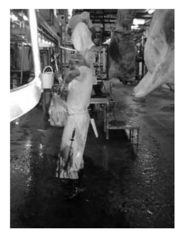
Figure 47: Lifting the head from the main rail to the head rail
