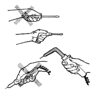
Figure 1: Deviated wrist position caused by design of the tool and its use. Wrist angle better (neutral) with the change in tool design (figures from Anderson, 1990)
