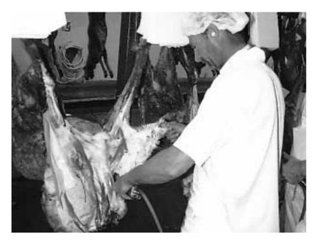
Figure 40: Using an air knife on the slaughter floor
