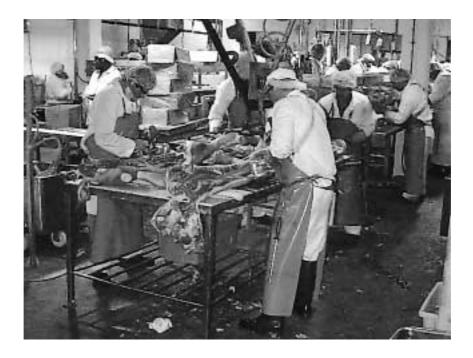
Figure 13: Heavier manual handling required on the cut up table compared to other tasks in the boning room
