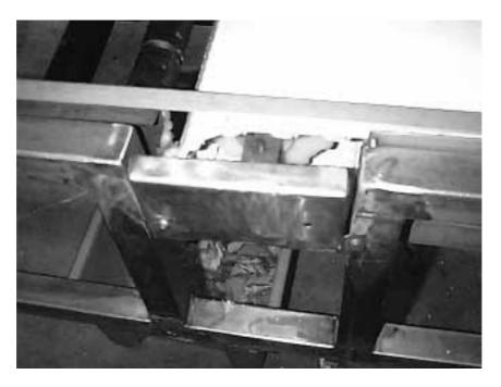
Figure 36: Exposed moving parts at the end of a packing belt
