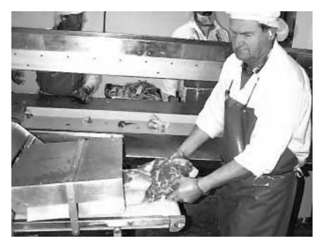
Figure 4: The de-rinder machine running parallel to the belt.
