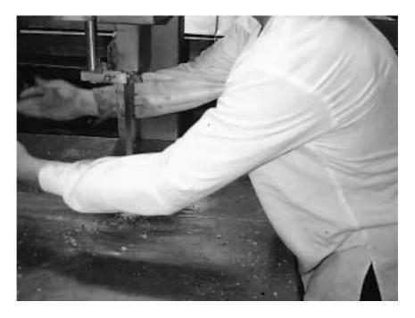
Figure 33: Pushing the carcass through the bandsaw requires the arms to travel past the blade up to the elbow of the operator
