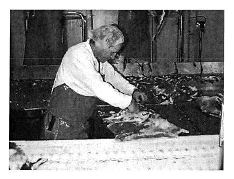
Figure 3: Slicing workstations that are set at different heights. The shape of the table also reduces the reach to the belt (Figure courtesy of Greens Meat Works, WA)
