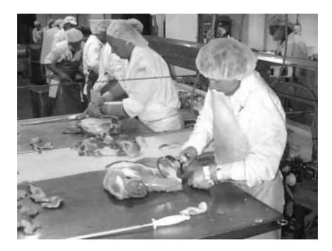
Figure 14: Lighter slicing tasks. Rotating between this task and heavier boning tasks can reduce the overall muscle load that is accumulated during the shift
