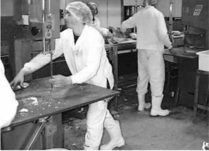
Figure 34: Using the bandsaw to cut the carcass
