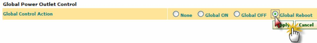
PS: All outlets that are turned on will reboot. Outlets that are turned off will remain as is. Each outlet will reboot with a delay of 'Sequence Timer' + 'On Power Failure Outlet Startup' seconds.
