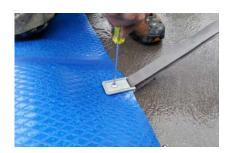
Fix the end of the strap onto a clean surface of the tube using the screws and washers provided.
