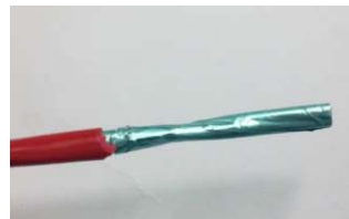
Cable Stripped of Fire Rated Insulation SHOWING RF Shielding
