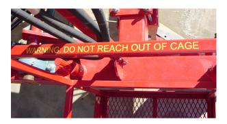
The operators platform was designed to keep the operator safe while the machine is in use. The operator should never lean over the platform to reach or grab anything while the machine is in use. The operator should always fasten the safety chain when on the platform. The safety pins should always be in the mounting tubes to keep the basket from bouncing out while the operator is on the platform. Their should only be one operator on the platform except for training purposes.
