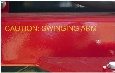
The operator should always remain on the operators platform until the swinging cone arms are completely open to prevent the operator from being struck by the swinging arm resulting in injury.
